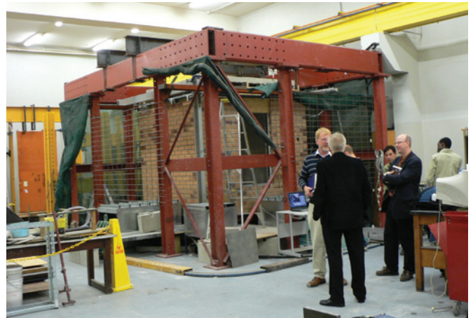
Test house on shaking table prior to test.
