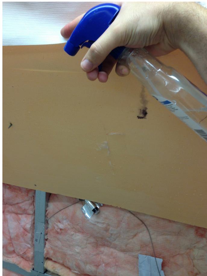
Figure B2. Spraying water to insulation batts and XPS foam
