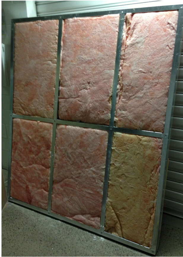
Figure 2: Steel frame with the insulation pink batts.
