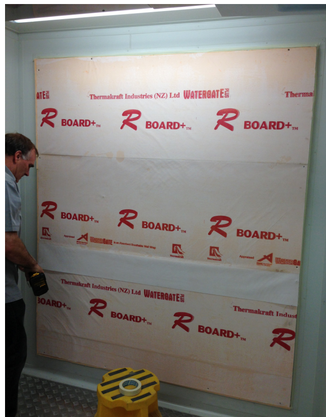
Figure 8: Photo of the wall test panel in the chamber.
